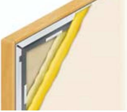
**An excellent sound barrier.** Cetra's acoustical panel is built over a solid inner partition covered with two layers of fiberglass per side and the outer panel fabric.
